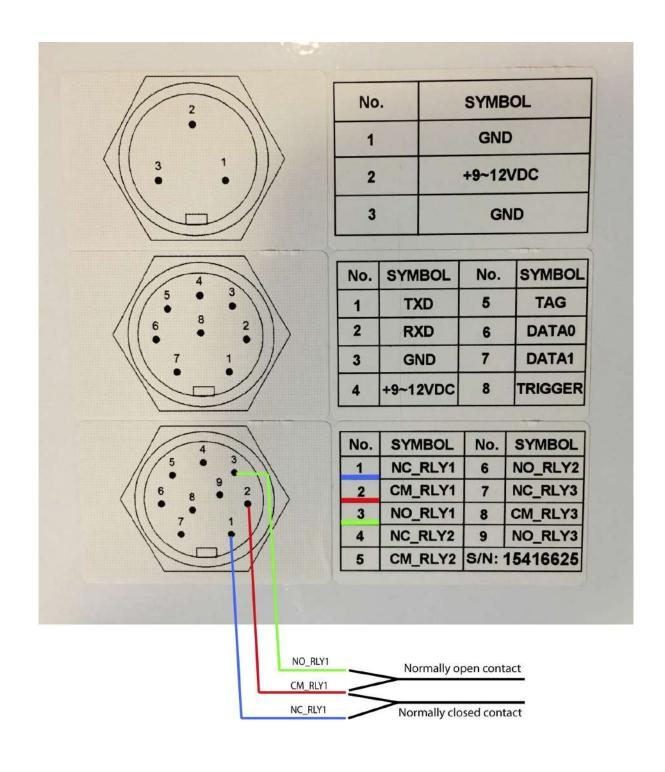
Connect with main controller(PC) by RS232 communication interface. The data format of RS232 interface is 8bits, 1 start bit and 1 stop bit, no parity bit; data rate can choose 9600, 19200, 38400, 57600 and 115200. RS232 communication interface support parameter configuration, demo program and serial communication secondary development kit function.
