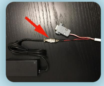
6) Antenna reader has additional settings such as power (tag reading range), frequency and tag binding code. To do this, you need to use the "Configurator" application for Windows OS. To connect the antenna reader to the computer, use the RS232 (COM) and USB adapter.
